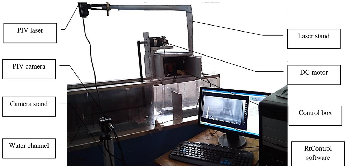
**Fig. 3:** A picture of PIV system setup and its connection to computer
